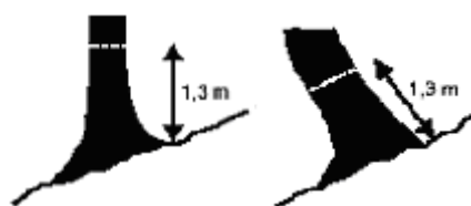
Figure (iv) Dbh measurement position for a tree on steep terrain.
